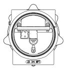
Figure 12-Terminal Strip Located Inside Wiring Compartment
