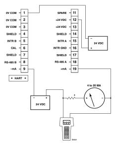
\*TOTAL LOOP RESISTANCE = 250 OHMS MINIMUM, 600 OHMS MAXIMUM. NOTE: SHIELDED CABLE RECOMMENDED (REQUIRED FOR ATEX).
