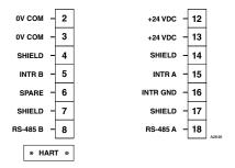
Figure 13—Transmitter Wiring Terminal Identification
