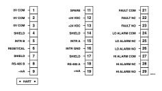
Figure 15—Wiring Terminal Identification for LS2000 Receiver with Relays
