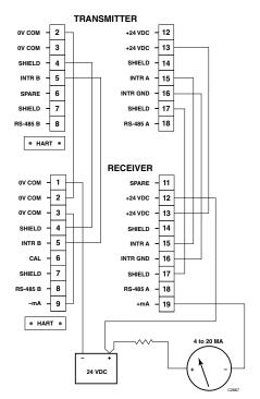
NOTE 1: TOTAL LOOP RESISTANCE OF 4-20 MA CIRCUIT = 250 OHMS MINIMUM, 600 OHMS MAXIMUM.
