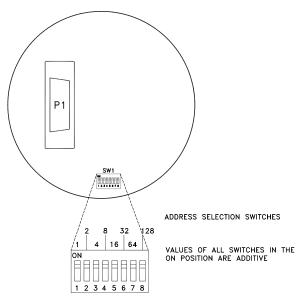
Figure G-2—Location of LS2000 Address Switches
