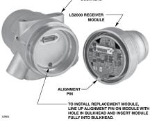
Figure 31—Receiver Module Removed from Bulkhead
