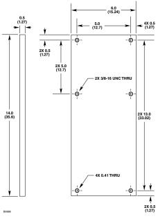
Figure 11—Dimensions of 012718-003 Flat Surface Mounting Plate in Inches (cm)
