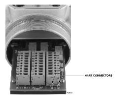
Figure 24—Location of HART Connector Pins (Receiver Module Shown) the cross hairs are centered on the window with the scope in both 180° positions.
